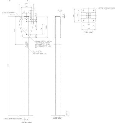
Recommended C20 grade of concrete in a 450 x 450 x 300 deep base.
